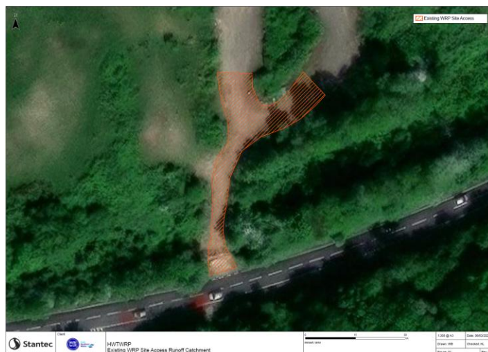
Figure 1 The Existing WRP Site Access Road Impermeable Area Catchment
